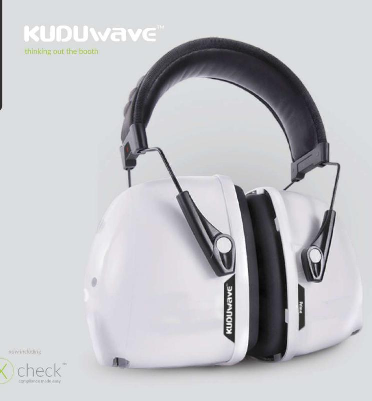
The KUDUwave Prime is a portable screening audiometer capable of audiometric testing without a sound booth.
